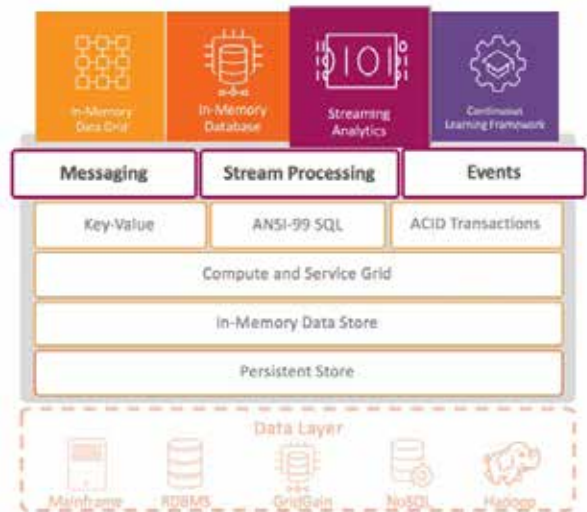
Figure 5. GridGain for Stream Ingestion, Processing and Analytics
