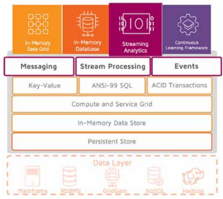
Figure 3. GridGain for Stream Ingestion, Processing, and Analytics
