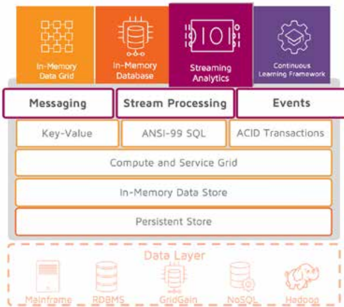
Figure 7. GridGain for Stream Ingestion, Processing, and Analytics
